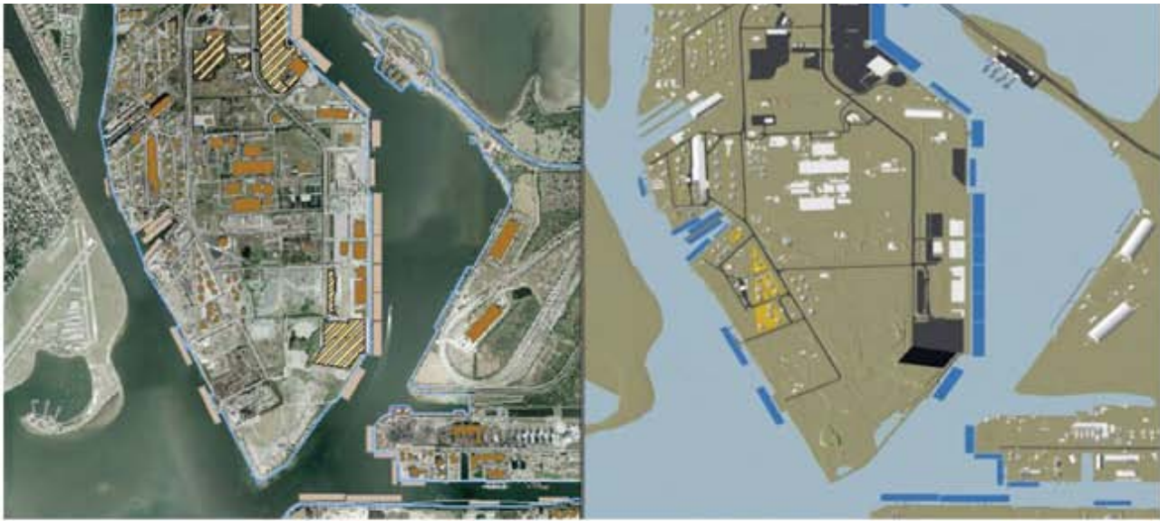
Three-dimensional framework data layers were developed for the Port of Tampa, Fla., from a combination of aerial mapping and terrestrial surveying methods.
