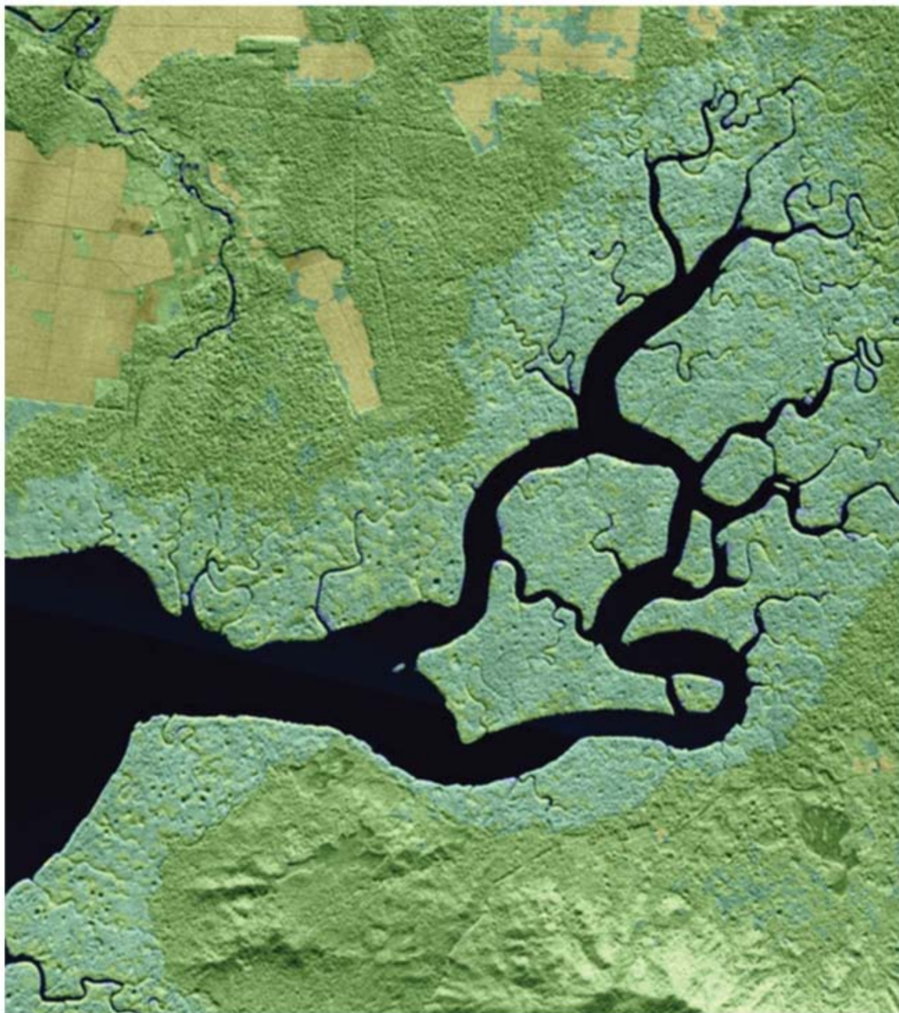
Fugro's GeoSAR airborne radar mapping system is used to accurately map littoral features and topography in equatorial regions that are difficult to map due to persistent cloud cover.
