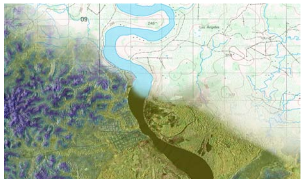
A topographic map with water features, roads, and forested areas identified blended with a thematic map generated from X- and P-band radar imagery.
